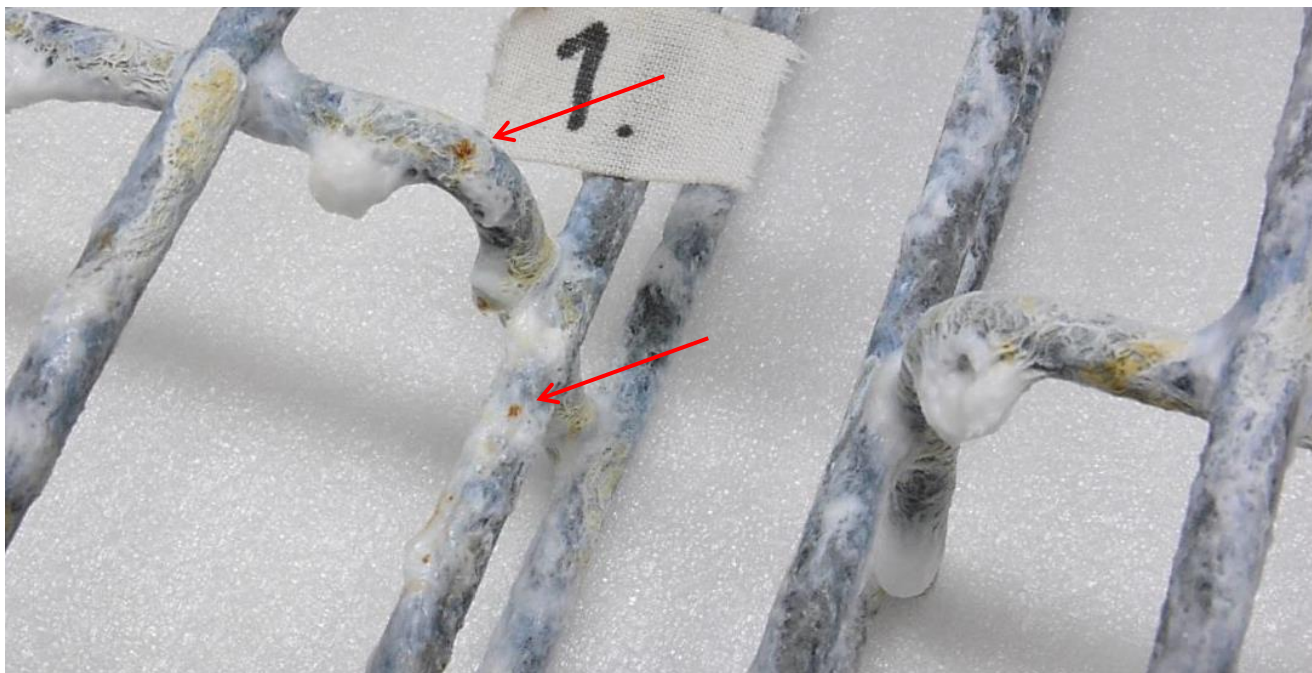
Picture 11. Close-up picture on sample 1 after 240h of testing. Example(s) of base metal corrosion is marked with arrow(s).
