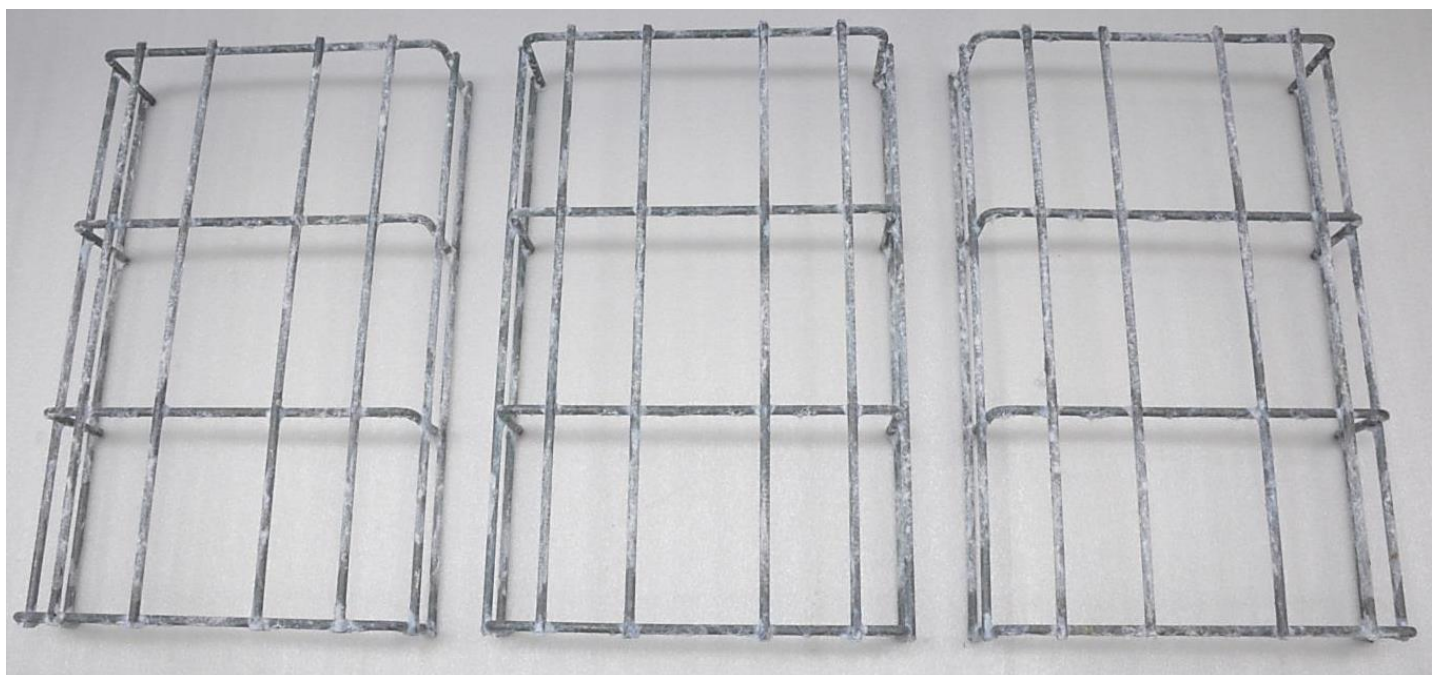
Picture 10. Samples 4-6 from the left after 240h of testing.
