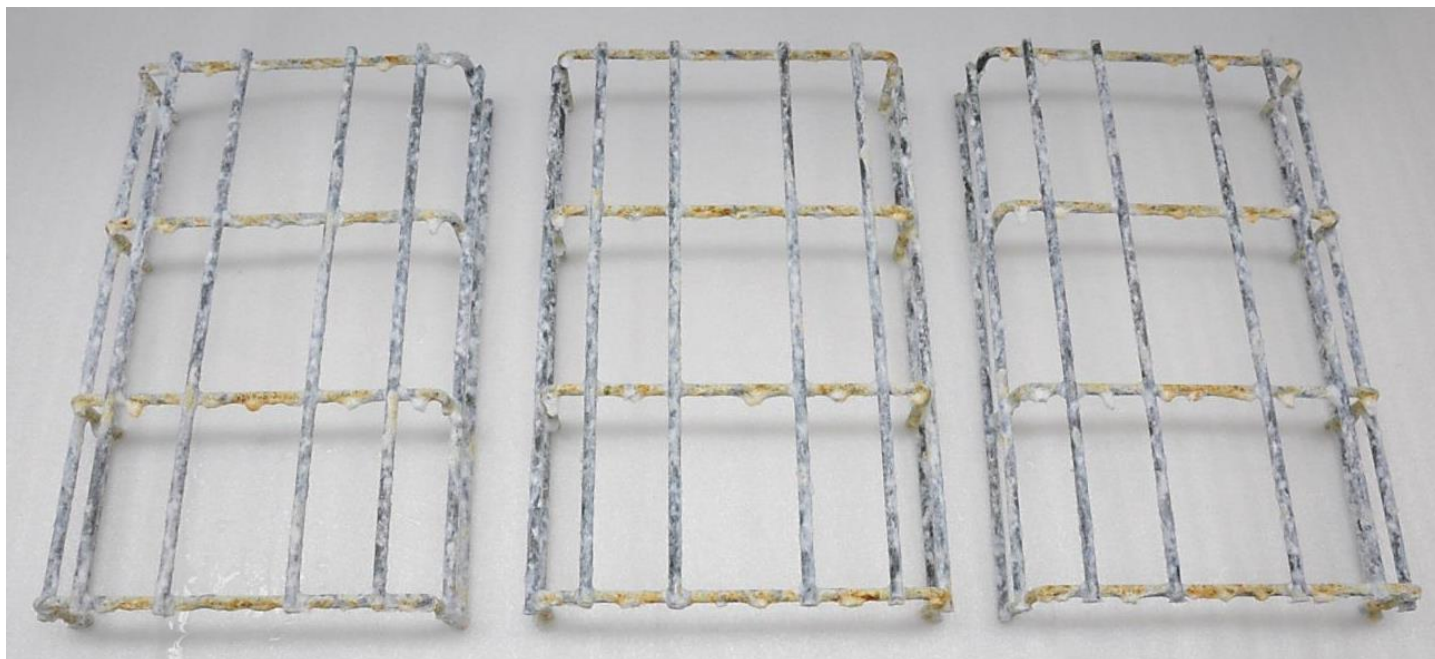
Picture 12. Samples 1-3 from the left after 504h of testing.
