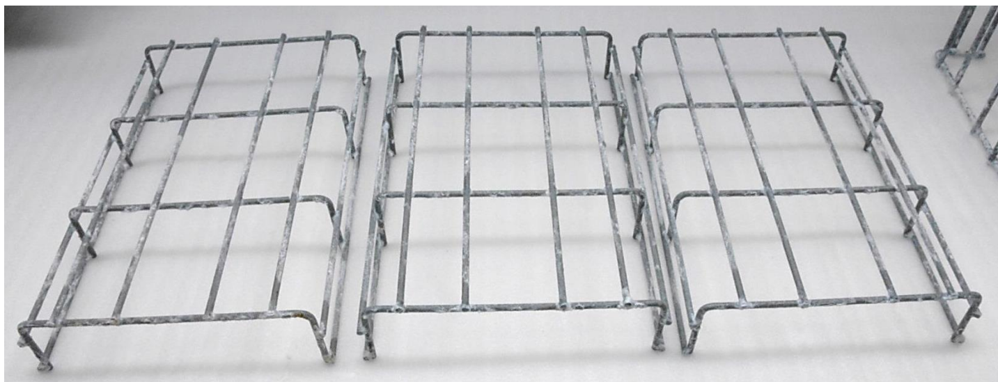
Picture 8. Samples 4-6 from the left after 168h of testing.
