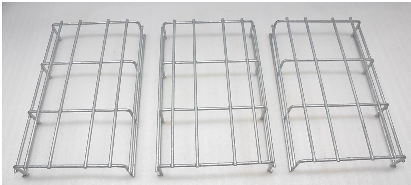
Picture 1. Samples 1-3 from the left before start of the corrosion resistance test.
