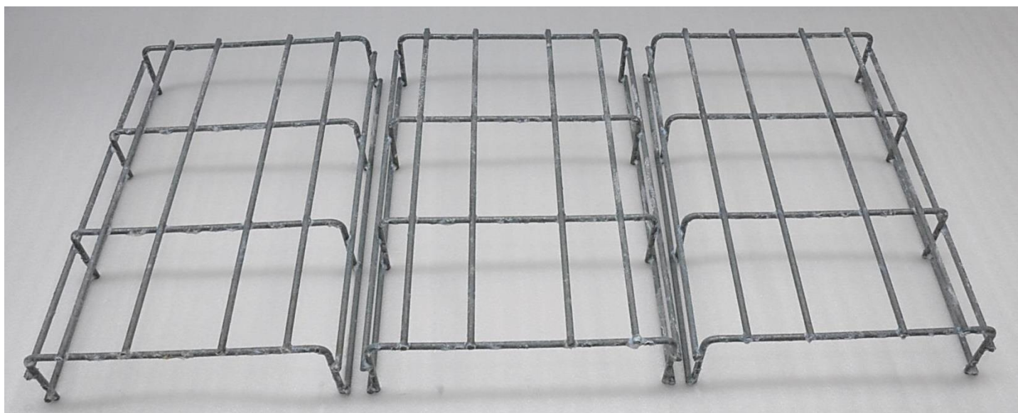
Picture 6. Samples 4-6 from the left after 96h of testing.
