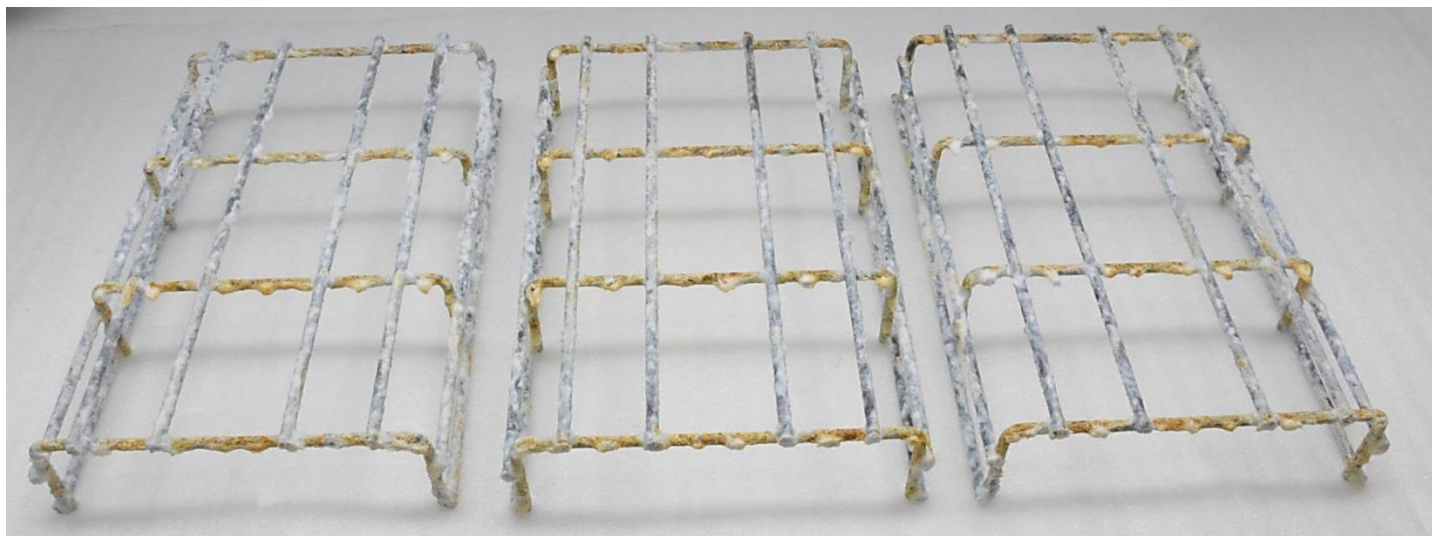
Picture 16. Samples 1-3 from the left after 744h of testing.
