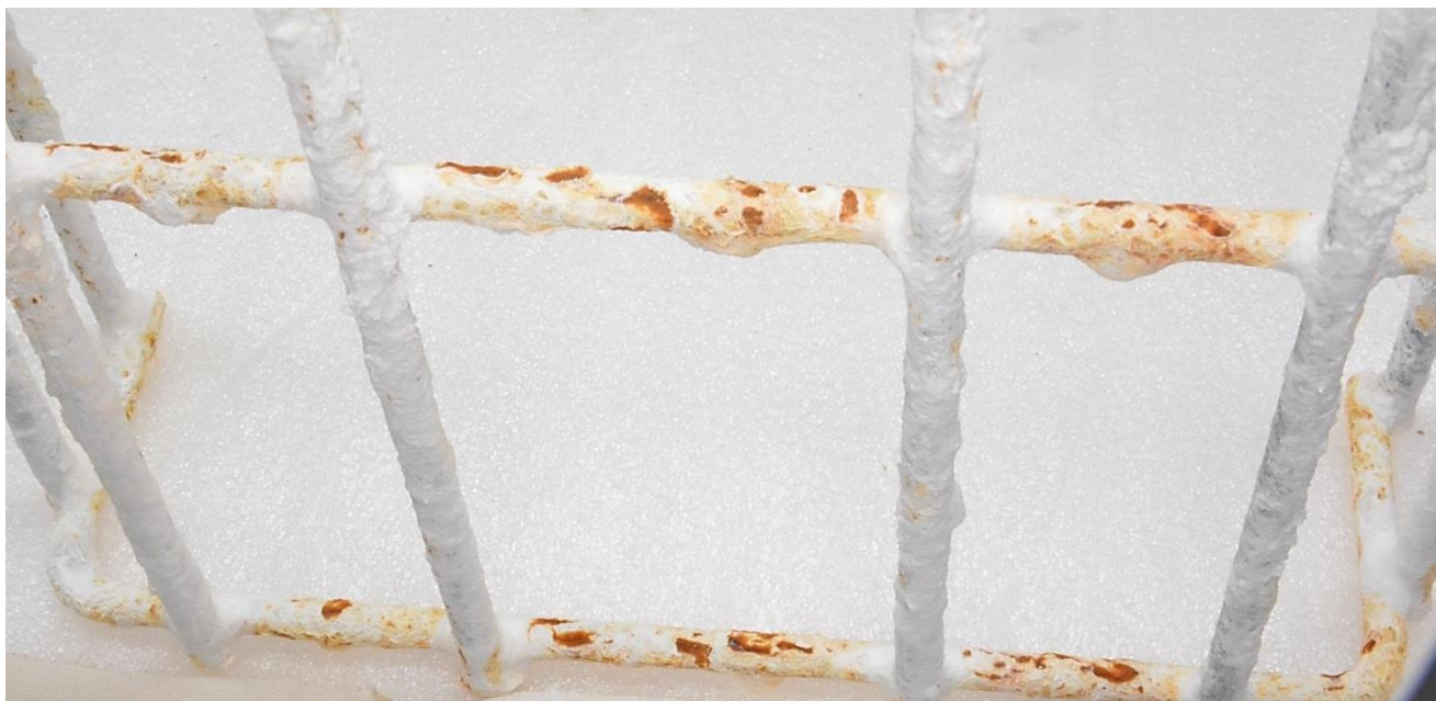
Picture 20. Close-up picture on sample 2 after 1008h of testing.
