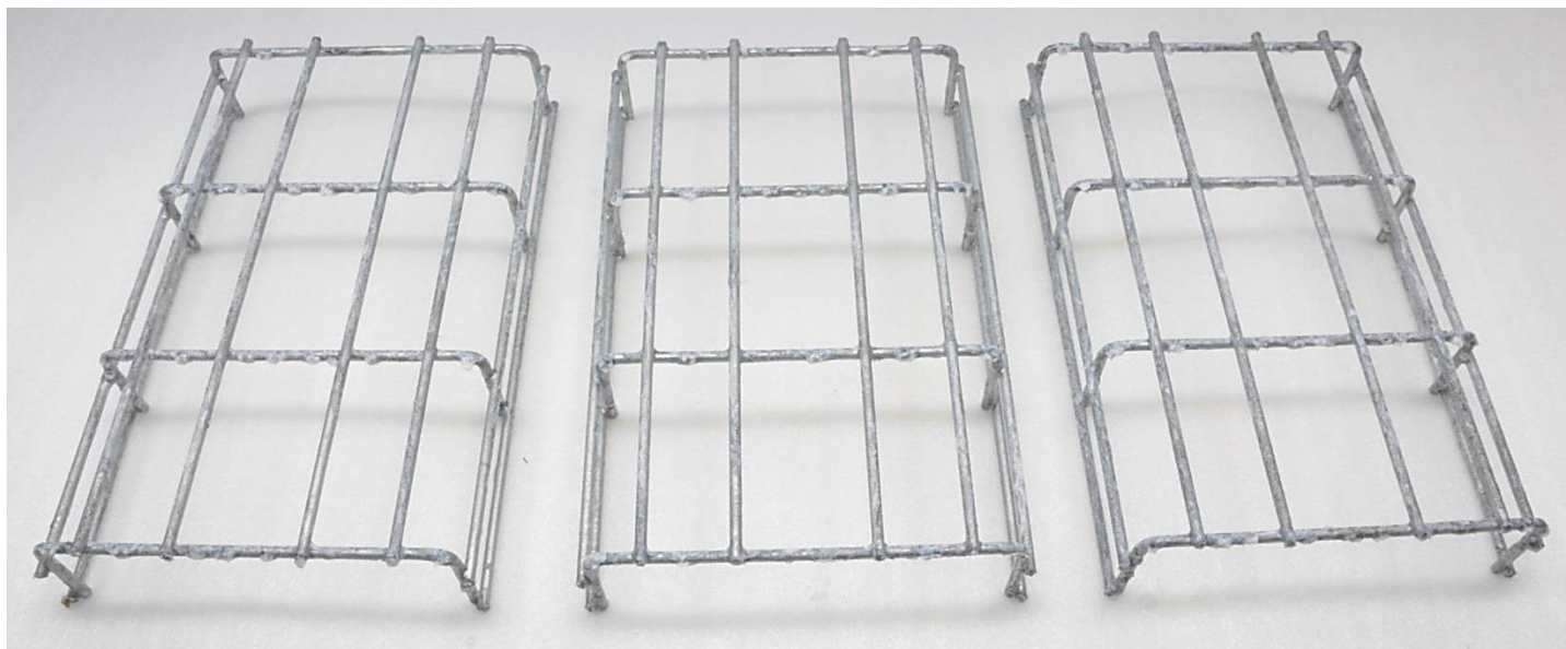
Picture 3. Samples 1-3 from the left after 24h of testing.
