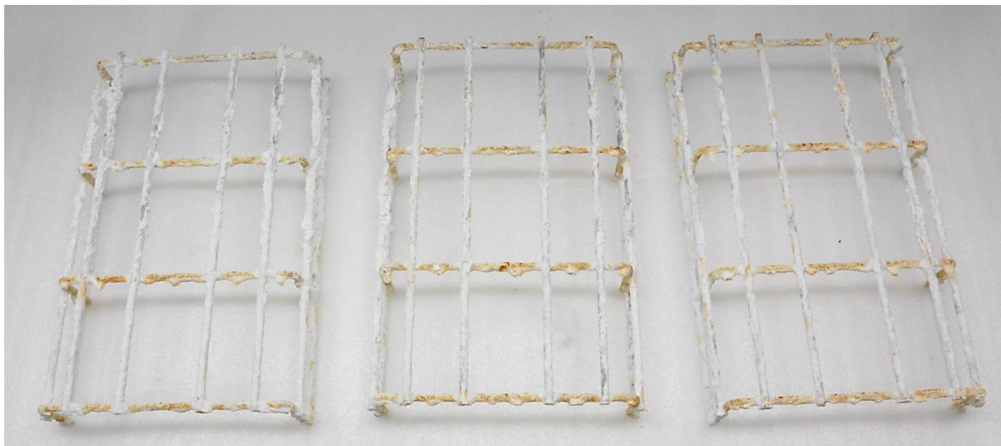
Picture 18. Samples 1-3 from the left when the test was finished after 1008h of testing.
