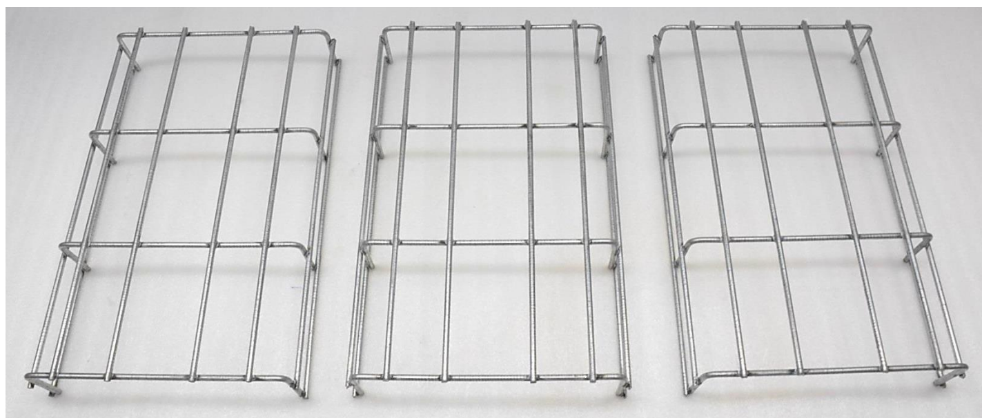
Picture 2. Samples 4-6 from the left before start of the corrosion resistance test.
