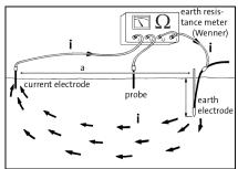
Measurement of earthing resistance - Method 1.
