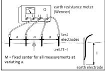
Measurement of earthing resistivity.
