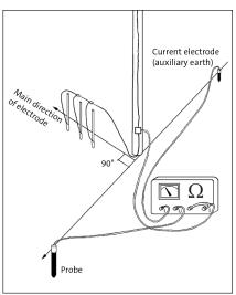
Measurement of earthing resistance -Method 2.
