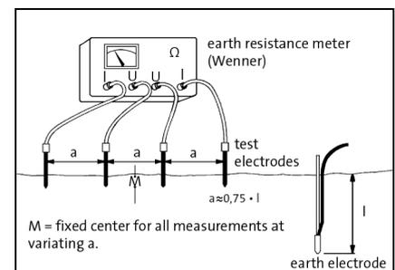
Measurement of earthing resistivity.
