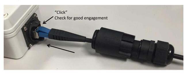
Remove the dust caps on the LC assembly and insert into the RRU. Listen for the sound of the latch engaging to insure a good connection.
