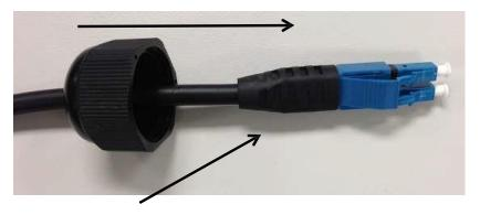
Feed the LC assembly through the backside of the cable gland nut in direction shown.
