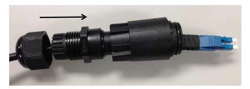
Slide cable gland nut over clamping fingers and tighten nut until slight resistance between cable gland and cable jacket. Note: The cable should still be able to move through the gland.
