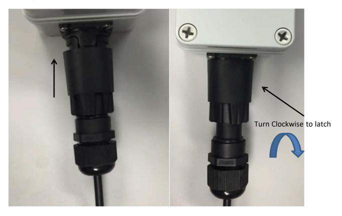
Slide the IP-RC to the RRU and turn the nut Clockwise to secure to bulkhead connector.
