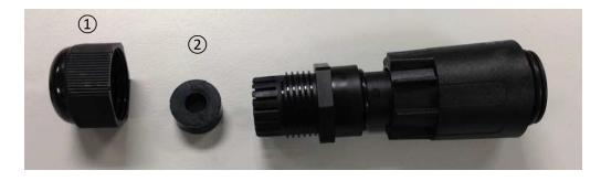
Remove cable gland nut ① and the split seal ② from the inside of the cable gland. Avoid using sharp or pointed tools that could potentially cause damage to the seal.
