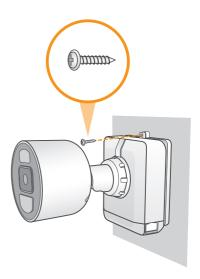
**OPTIONAL:** Tighten the pre-installed locking screw on the base of the Power Pack using the included screwdriver.
