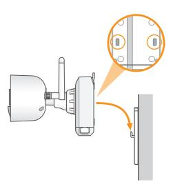
5 Insert the security screw through the fasteners on the top of the camera base and mounting bracket to secure the camera to the mounting bracket. Tighten using the included screwdriver.
