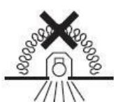
The luminaire is not suitable for covering with thermally insulated material
