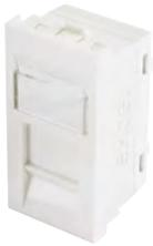
Excel Category 5e RJ45 modules comply with the EIA TIA Standard for enhanced Category 5. Each shuttered module is supplied with a slide label field and space above, this is allowed for use of self adhesive or further labelling if required. Termination can be made using LSA tooling, a cable tie base is positioned between the IDC blocks to relieve cable stress.
