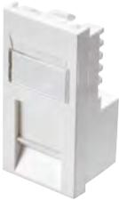
The Office Excel Category 5e Unscreened RJ45 low profile module has been designed to be used in conjunction with the Office Hardware Mounting Range. Excel Category 5e Low Profile RJ45 modules comply with the standards for enhanced Category 5. The product provides quick and easy termination using LSA compatible tooling. Port identification can be completed by use of the integral slide label or simple application of an adhesive icon.
