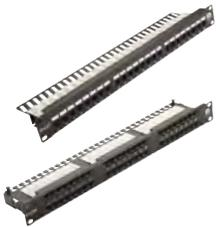
Available in 24 or 48 port options the Excel right angled patch panel represents a cost effective category 6 solution with integral rear cable management. Both occupy 1U position and present LSA compatible termination IDCs that are horizontal to the panel facia to allow quick and easy cable installation. The 48 port version uses a double deck design to facilitate two sets of 24 ports to be installed.
