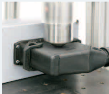
Impact of falling hammer weighing 1.7 kg
